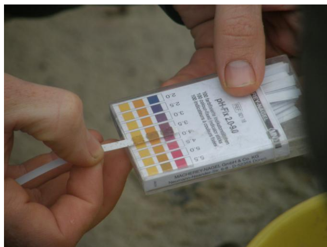
Acid sulphate soil test result at Point Sturt – about 3.5!
